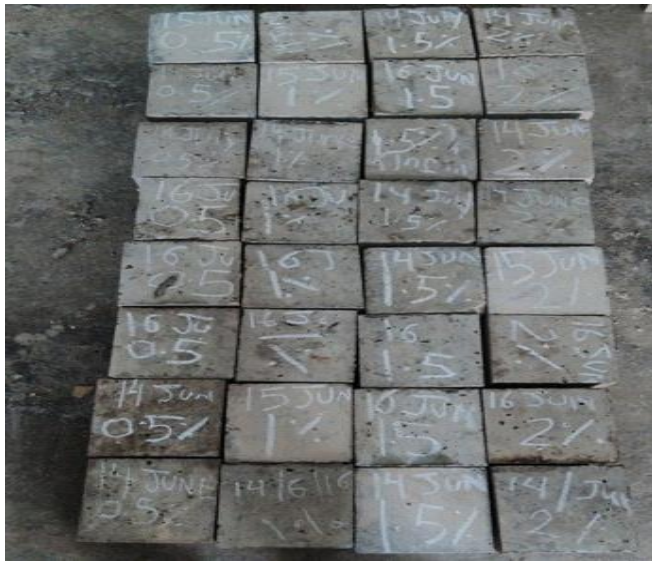
Procedure for compressive Strength Test of Geopolymer Concrete Cube
