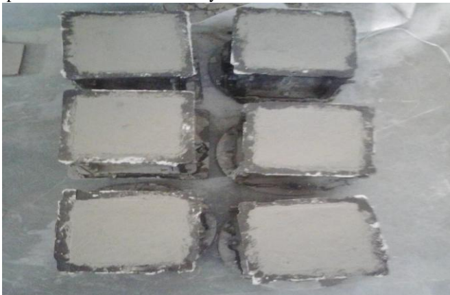
Fig. 3.3 (a): concrete cubes casted in the mould
