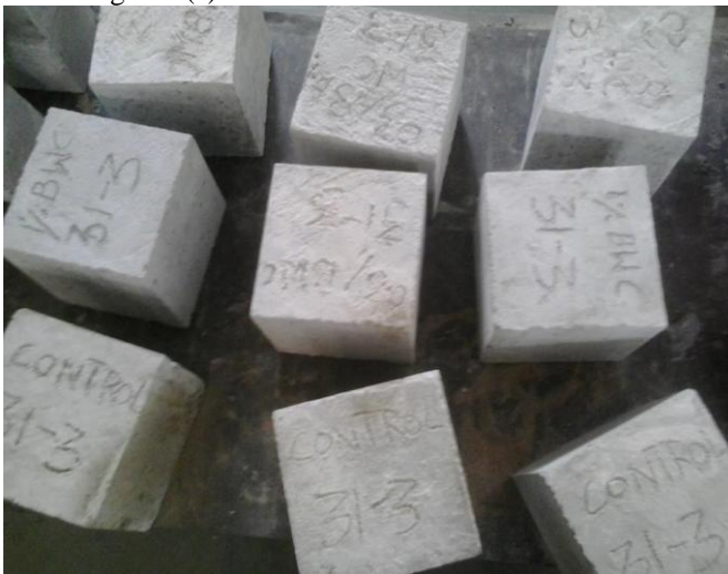
Fig. 3.3 (b): concrete cubes after de-moulding Fig. 3.3: (a) and (b) shows some concrete specimen cast in laboratory
