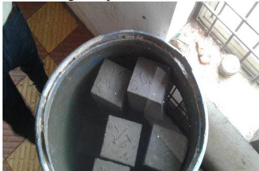
Fig.5 Curing of cubes
