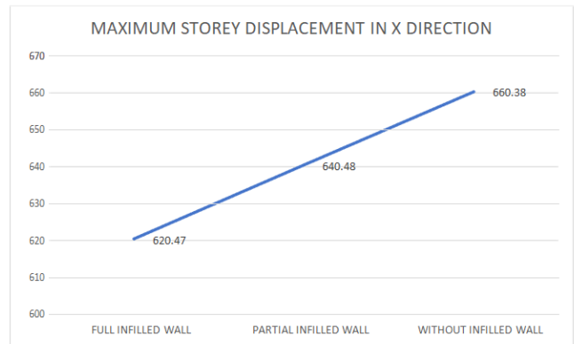
Fig. Figure showing maximum storey displacement in X direction in zone V in the structures
