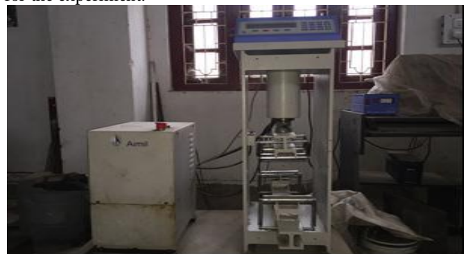
Figure 3.2 Flexural testing machine for Geo-polymer concrete
