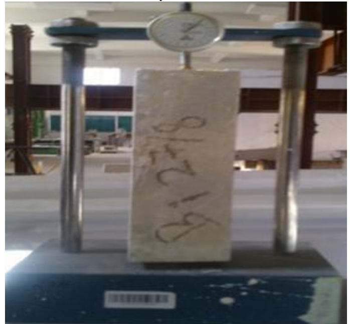
Figure 3.4 Drying shrinkage test for Geo-polymer concrete
