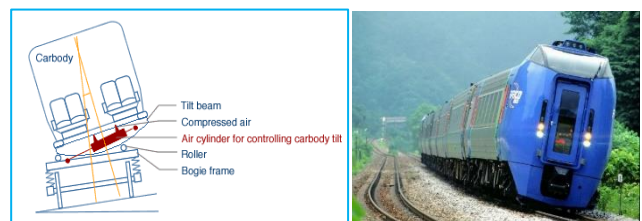
Fig. 5. Tilting train mechanism
