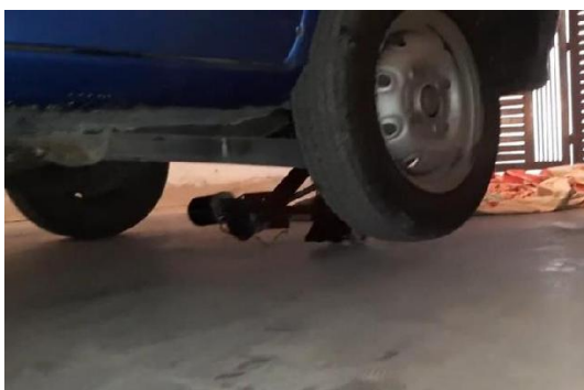
Fig. 6 Movable Jack lifting Maruti 800
