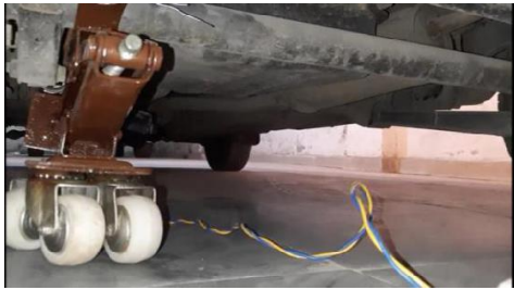
Fig. 5 permanently installed jack beneath The automobile (In extended position)
