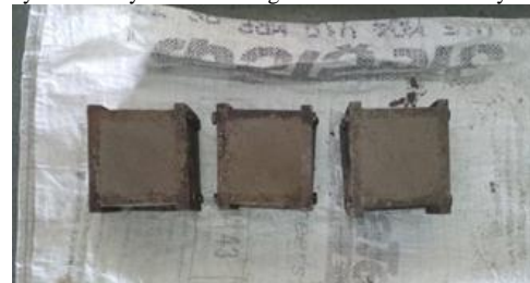
Figure Test Samples of Fly Ash Mortar
