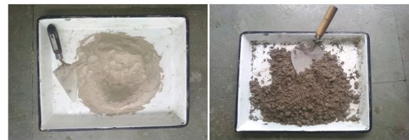
Figure Dry Mix of Fly Ash Mortar Figure 3.19: Wet Mix of Fly Ash Mortar
