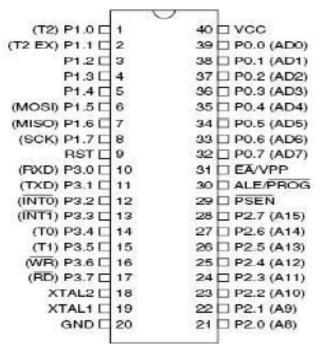
Fig .9. Pin Diagram of AT89S52
