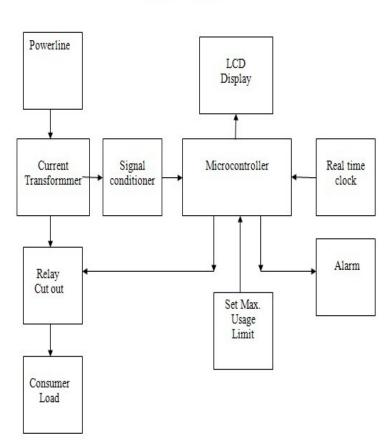
Fig. 1. Operational block diagram of remote data acquisition using wireless SCADA system
