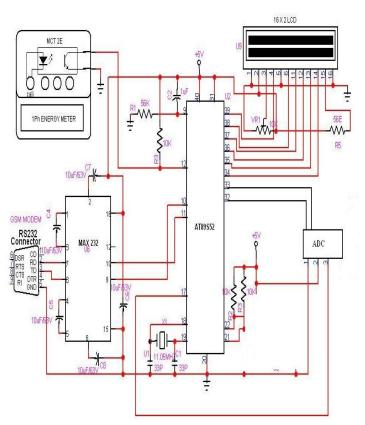
Fig .10. Circuit flow of the entire process
