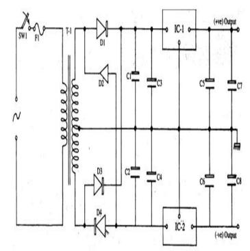
Fig. 3. Circuit diagram of full wave regulated power supply using IC's
