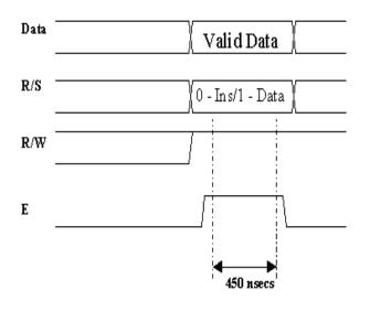
LCD Data Write Waveform
