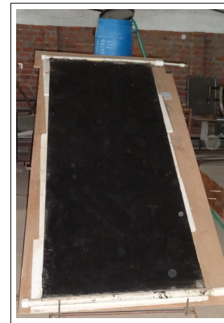
Figure 2: Actual Experimental Setup of Polycarbonate Collector based solar water heating system.
