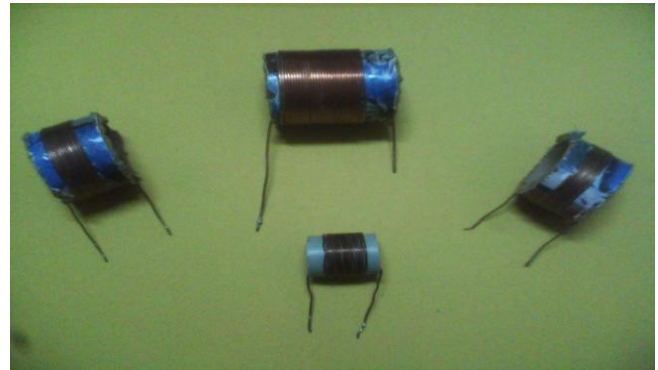
Fig.4. Copper coils wound on cardboard with air core
