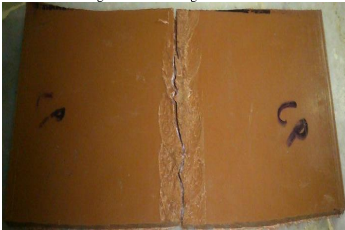
Fig. 3. The tensile test fractured specimen
