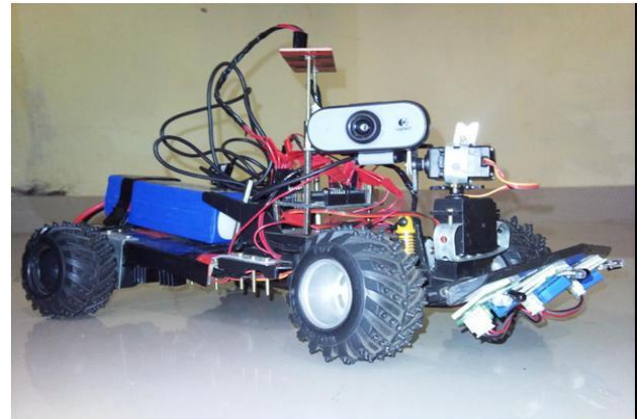
Fig. 4. Prototype command controlled unmanned ground vehicle (UGV)
