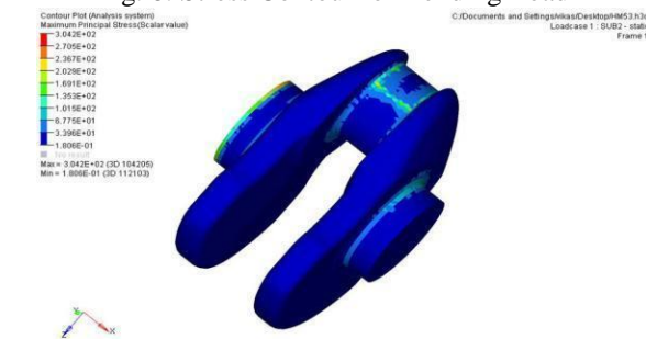
Fig. 9: Stress C o n t o u r for Torsional Load
