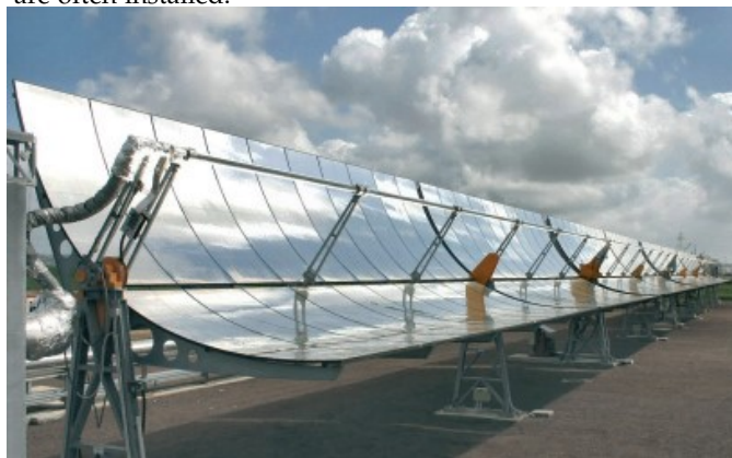
Figure 1: CSP Parabolic Trough Solar Collectors
