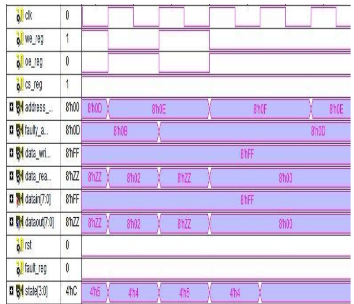
Fig 4.Detection of faulty address 11 and 13
