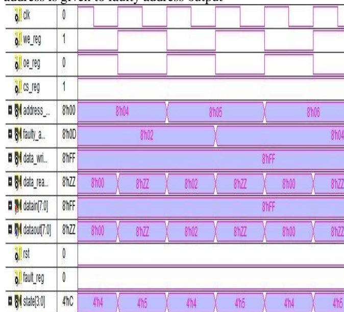
Fig 2.Detection of faulty address rows 2 and 4
