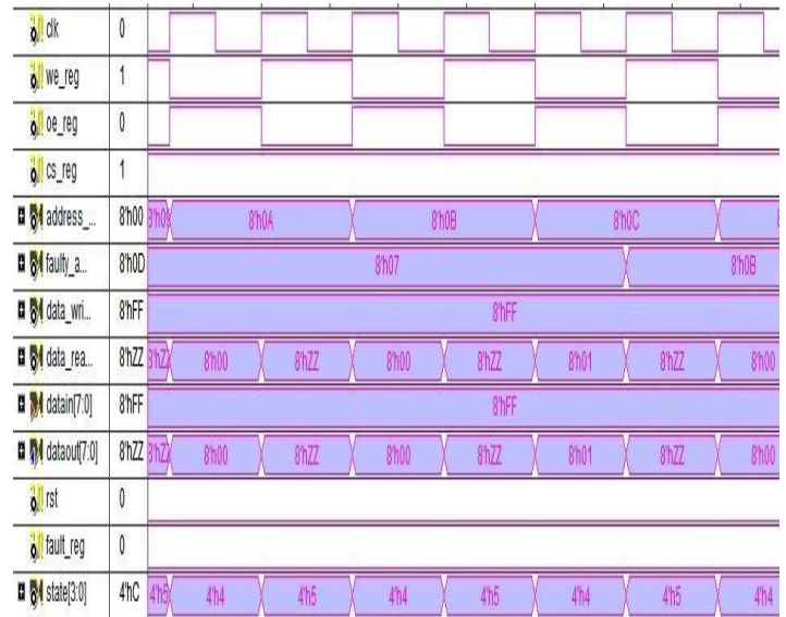
Fig 3. Detection of faulty address rows 7 and 11
