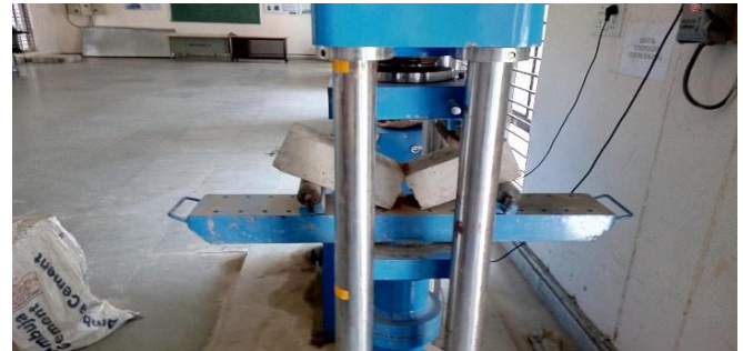
Figure 7 flexural test on concrete beam
