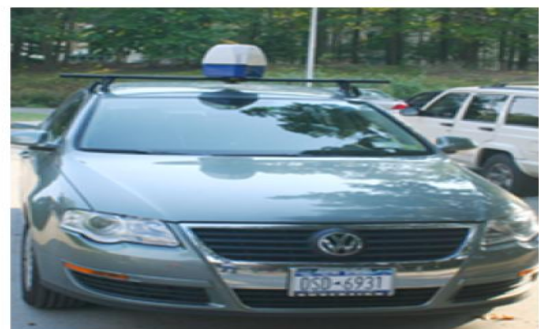
Figure 7: Antenna mounted on top of car to enhance network connectivity
