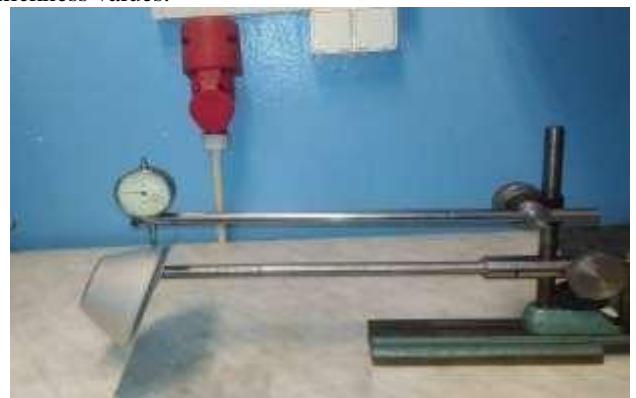
Fig. 7 Thickness measurement at different heights of formed sheet metal
