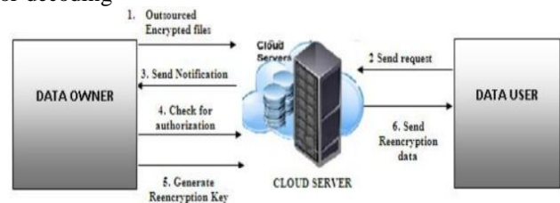
Fig: System architecture for Security Enhancement of Cloud Data Storage Using Identity Based Encryption
