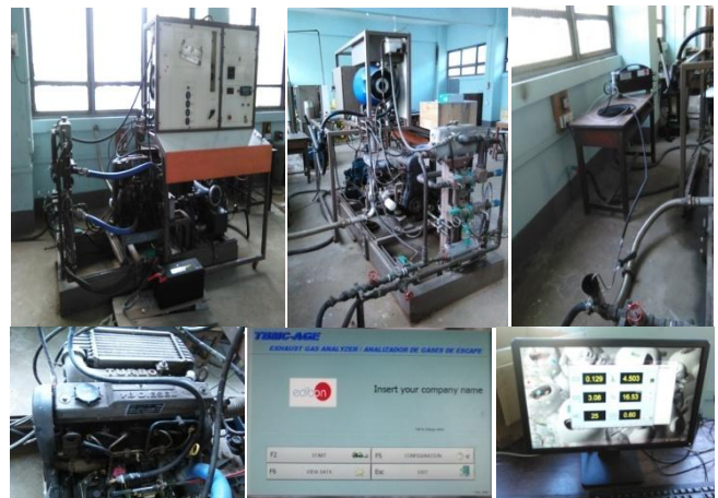
Fig. 2. Turbocharged Diesel Engine Test Bed with Exhaust Analyzer
