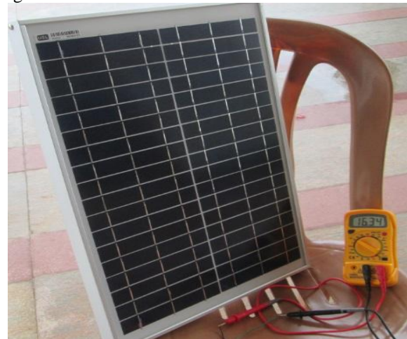
Fig. 12. Setup of 20W, 16V solar panel
