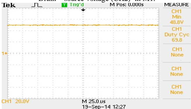
Fig. 15. Output voltage of solar powered IDBB The efficiency of the solar powered IDBB converter is 84-85%.
