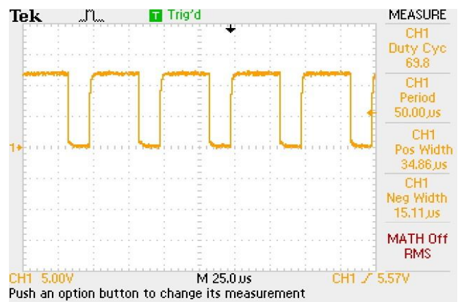
Fig. 13. Waveforms of gating pulses for MOSFET switch M1.
