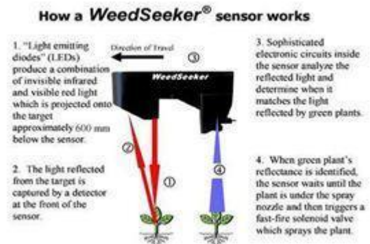
Figure 6: How weed seeker works
