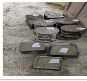
Figure-6 Steel Molds with concrete
