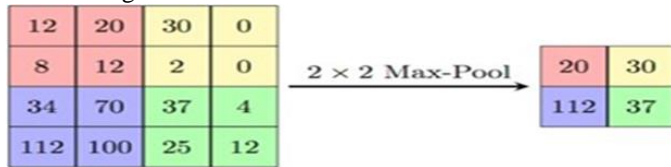
Figure 3. describes the max-pooling from the 2*2 window and reducing the dimension
