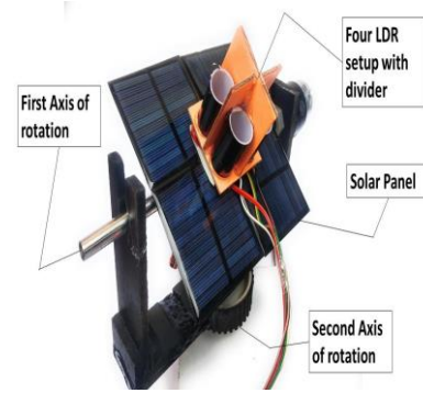
Fig. 7: Hardware Assembly of Solar Panel
