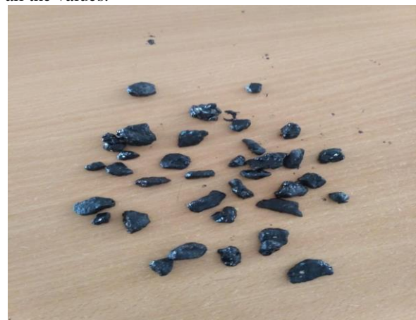
Figure 2. Aggregates after stripping test with addition of Hydrated lime
