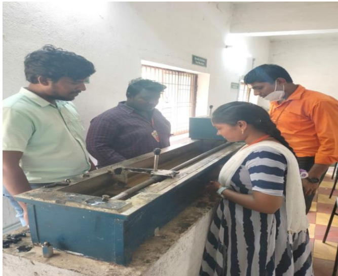
Figure 2. Ductility testing of Bitumen
