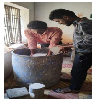
Fig .5: curing of cubes.
