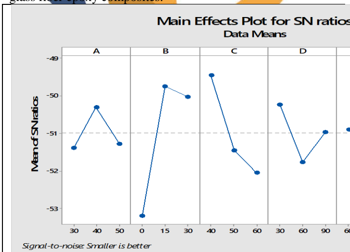
Fig. 5.1 Effect of control factors on erosion wear rate of glass fiber-epoxy composites
