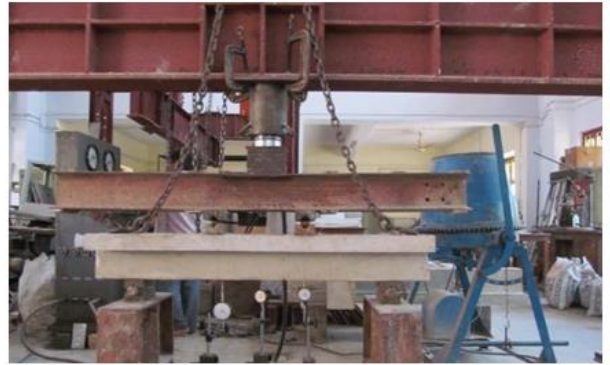
3 (a) Experimental Setup of beam Solid beam
