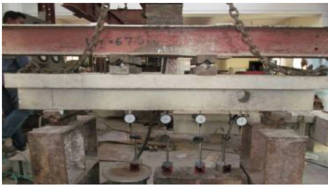
4(a) Experimental Setup of the CBA under four-point loading
