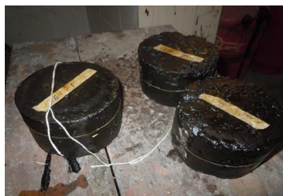
Fig 4.6- Sample after Paraffin wax Coating
