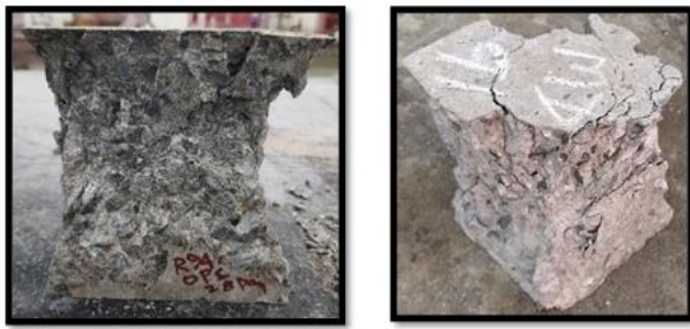
Figure 4.2. Brittle failure of cubes under compression
