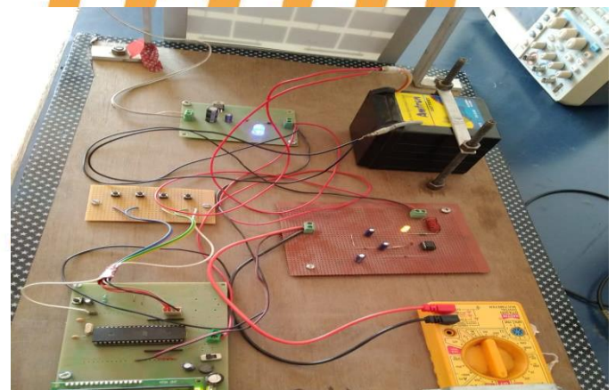
Fig.16- Solar PV System with Boost Converter
