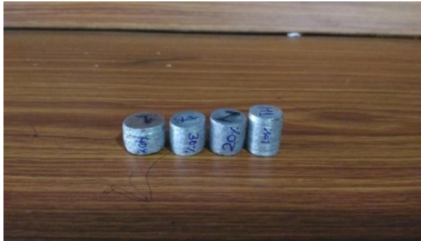
Figure 3.8 Composite specimens showing bulge profiles at various deformation stages under compression testing
