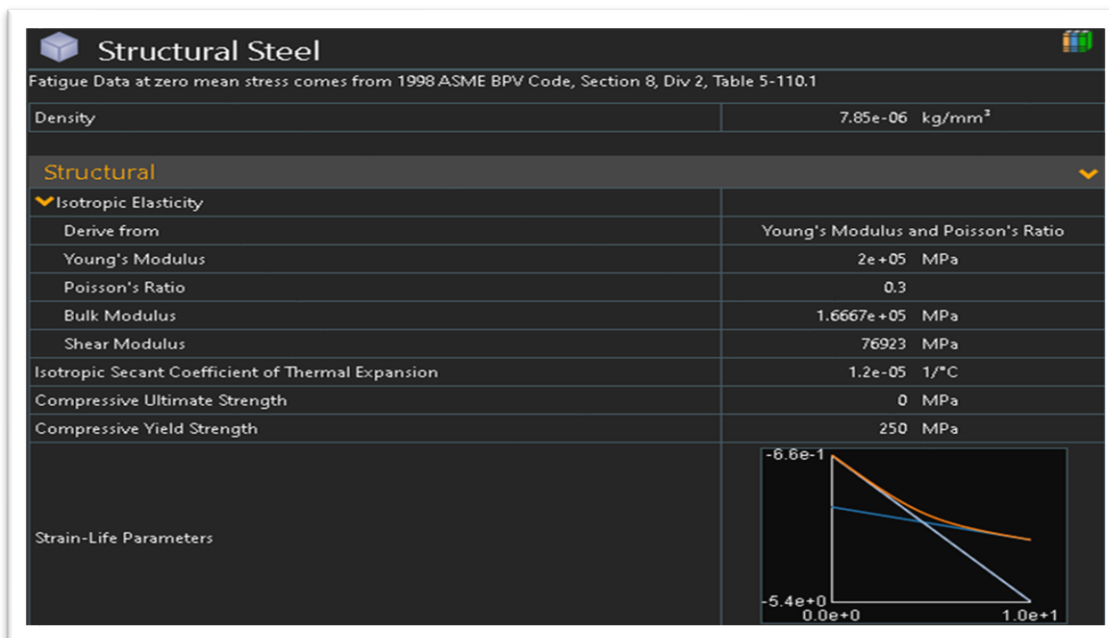
Figure.6.5 Structural steel property
