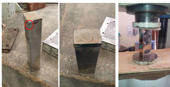
Fig. 15 Failure in Filled Section
