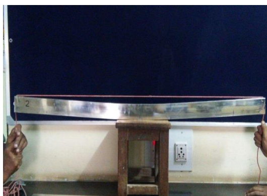
Fig 11 Bending at mid span in In-filled specimen. Note: No crimping nearpoints of load application
