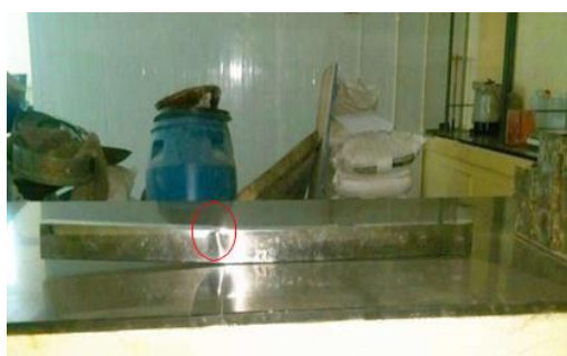
Fig 12 Local buckling of hollow specimen
