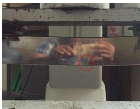
Fig 13 Failure crack in In-filled Specimen
