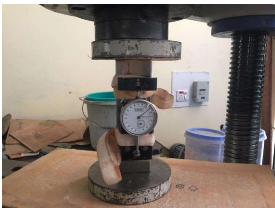
Fig. 14 Experimental set-up for compression testing.
