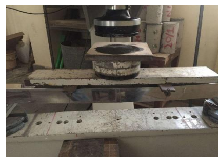
Fig 9 Specimen after removal of load.
