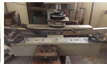
Fig. 8 Bending of the specimen.
