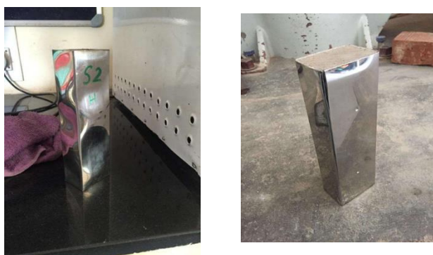
Fig 16 Buckling of Specimen Fig 17 Splitting of Specimen
