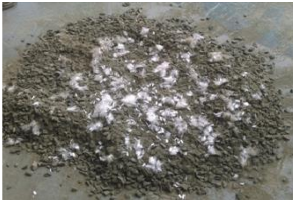
Fig. 3.2 Addition of polypropylene fiber
