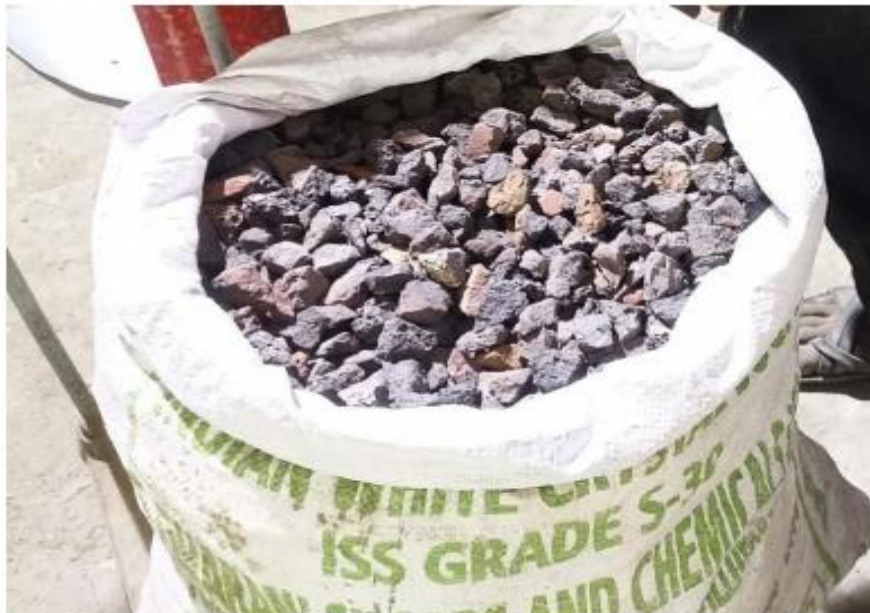
Fig.1.2 Crushed Over Burnt Clay Bricks
