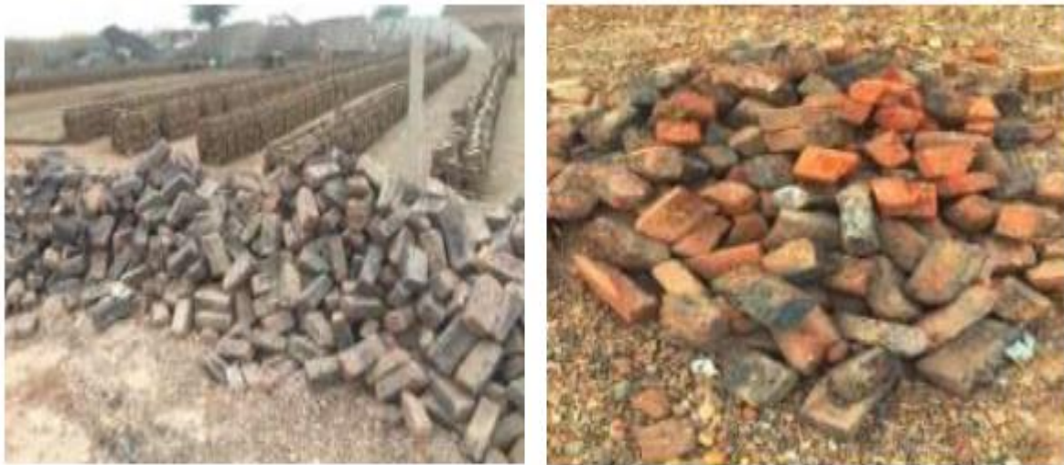
Fig.1.1 Over Burnt Bricks as Construction Waste
